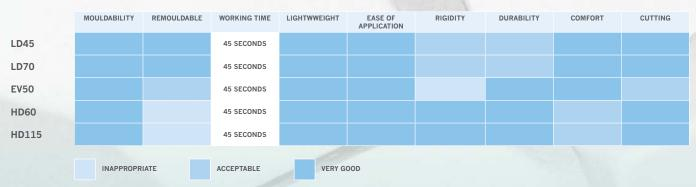
Guide 'working times' are based on 6mm thick material for HDPE grades and 12mm thick material for other grades. The product range is constantly being updated; new colours, new densities or more specialist foam grades. Full information on request.
